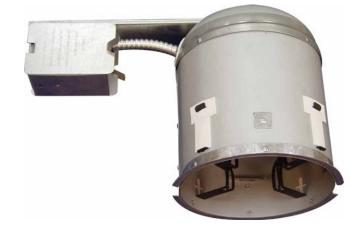
V8667 6 inch Remodel Recessed can IC , Air Tight, 90W Thermally protected housing Adjustable socket bracket Wire through junction box (2 in and 2 out) Adjustable hanger bar from 14" to 24" Spring clips for fast and easy installation May be covered with insulation Housing adjusts for ceiling up to 1" thick Suitable for damp locations Commercial or residential
